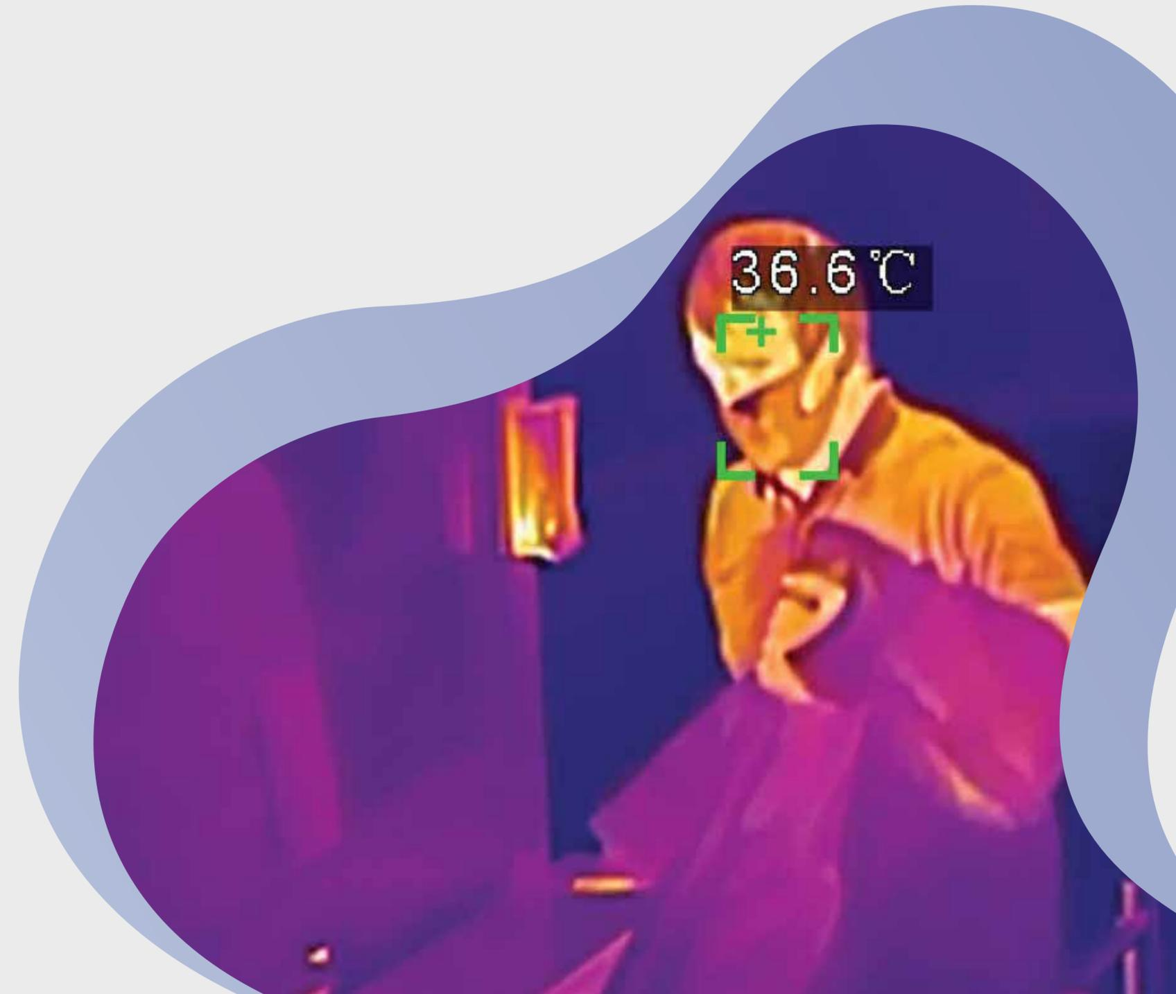
The VideoNet Defender Thermo complex is designed for remote recognition of a person by face, non-contact measurement of their temperature, with automatic logging of the event series and saving data for subsequent analysis, in the following format:
